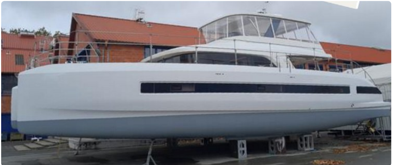
Freshly painted hull (Awlgrip) – photographed at the yard
